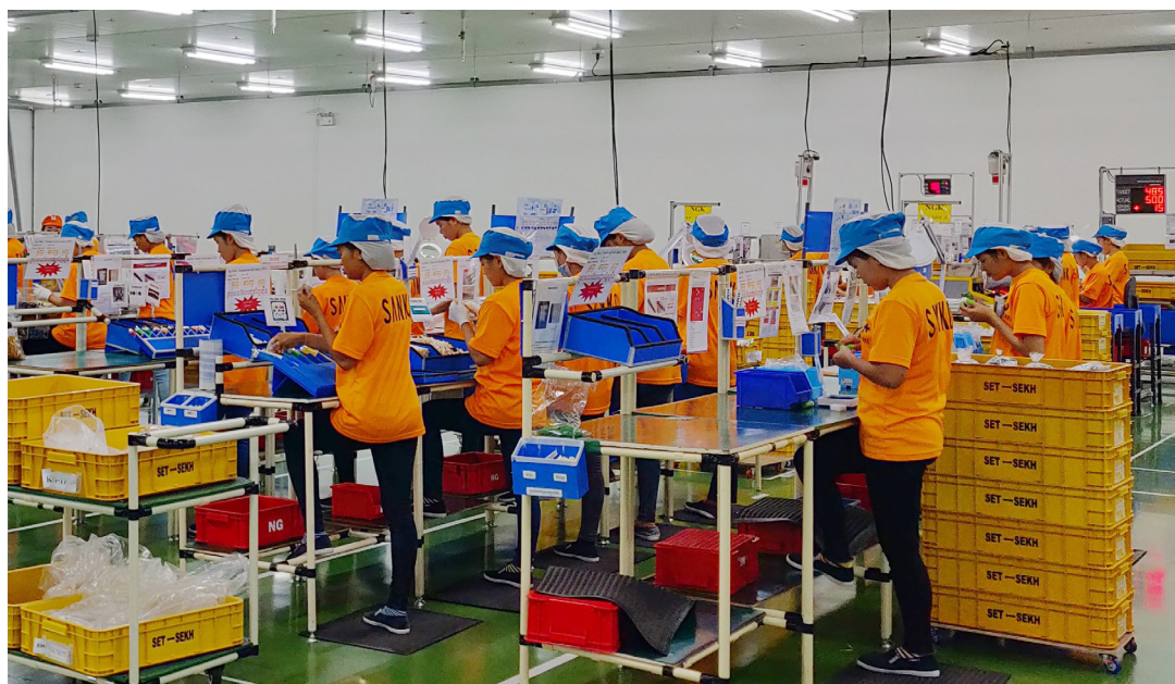
Assembly line workers producing wire harness in an electrical and electronics factory, Banteay Meanchey, January 2022
